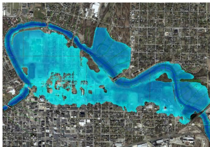
Fig-2: An integrated 1D-2D flood model showing flood conditions in a city area using HEC-RAS
