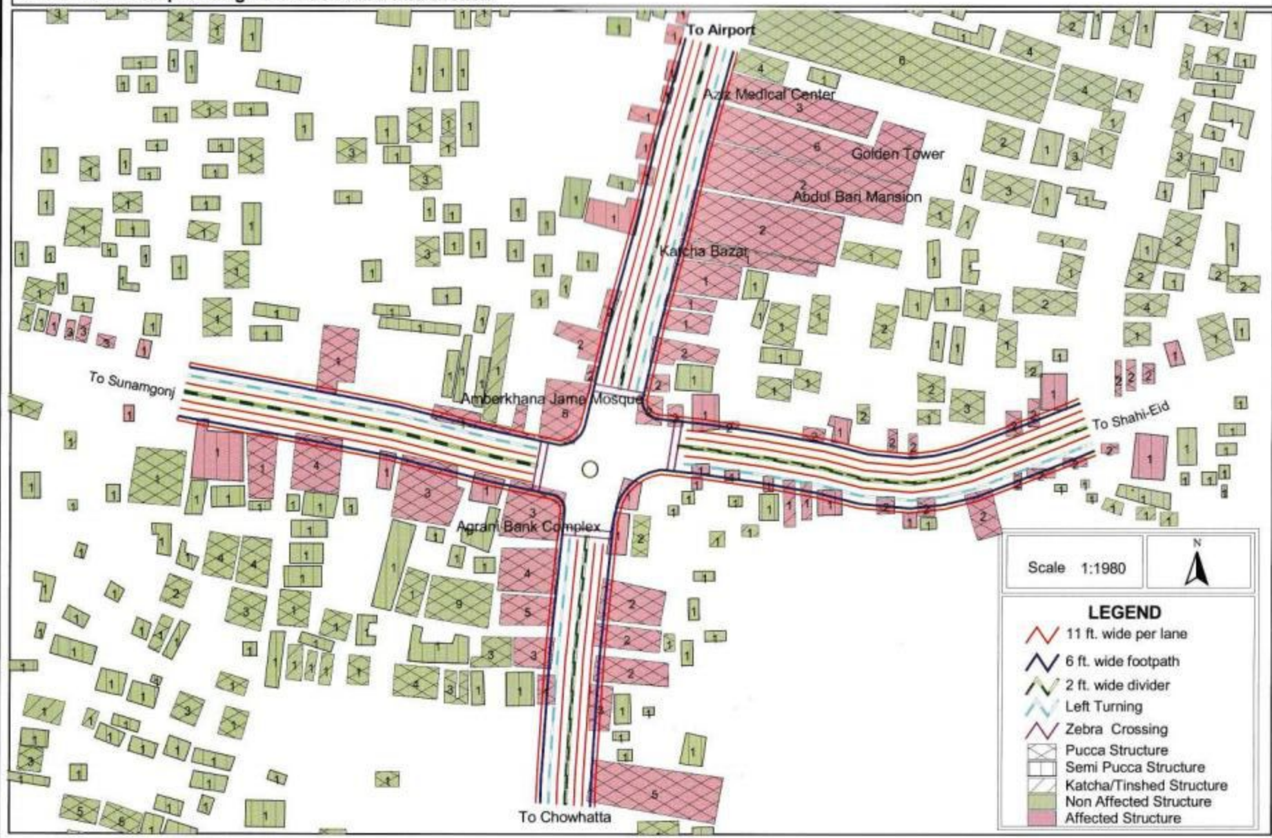
Annex: 1.3a: Sample Design of Amberkhana Intersection
