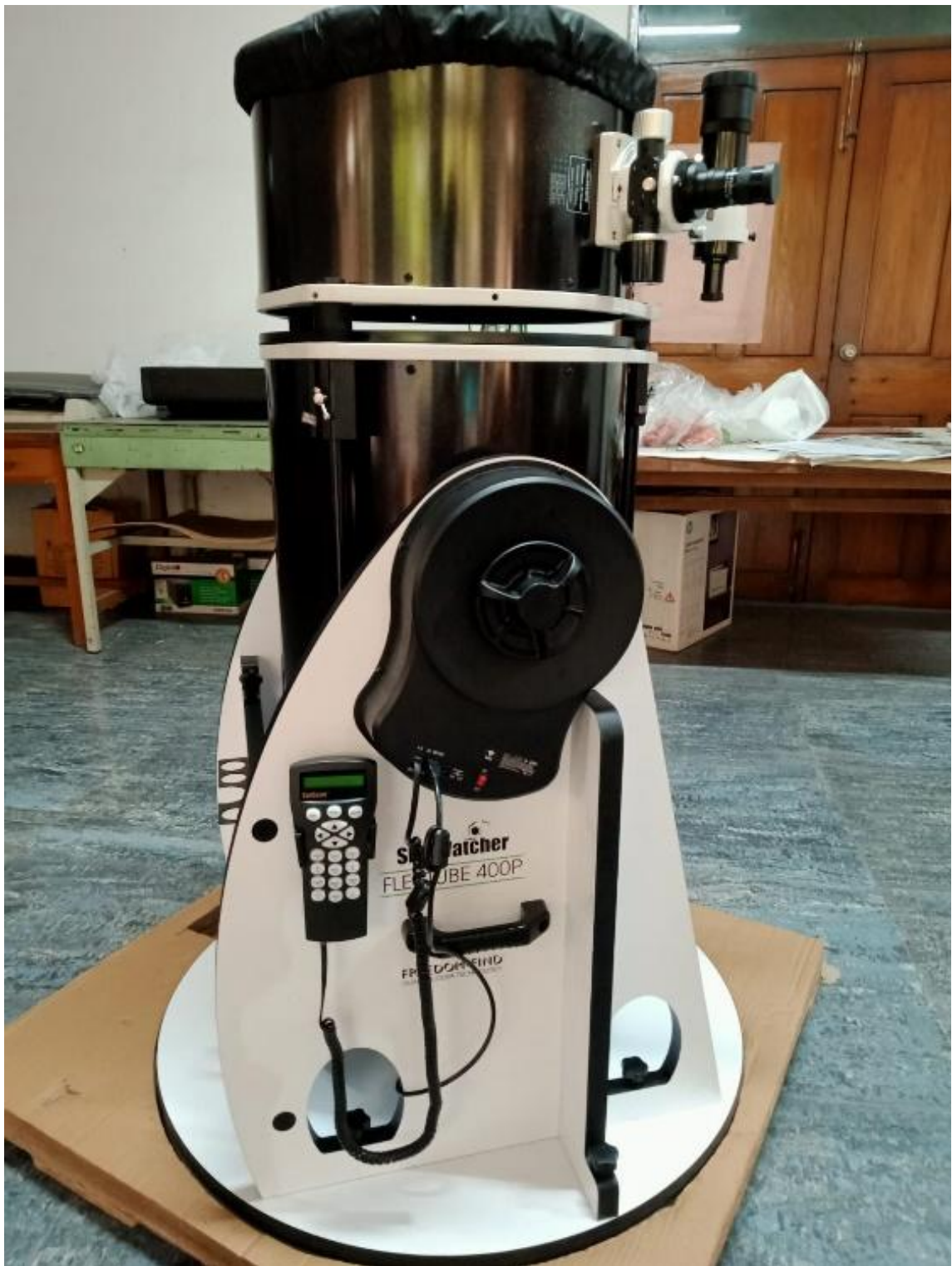
Fig. 2.7.4 Optical Telescope: 16-inch/ 400 mm Sky-Watcher Dobsonian Reflector Telescope
