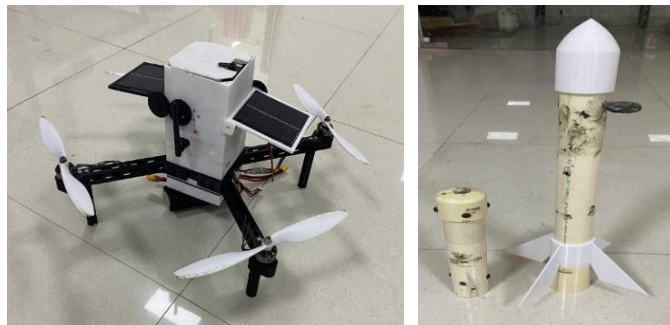
Fig.2.9.2: Assembled CubeSat and Rocket with solid rocket motor & rocket nozzle
