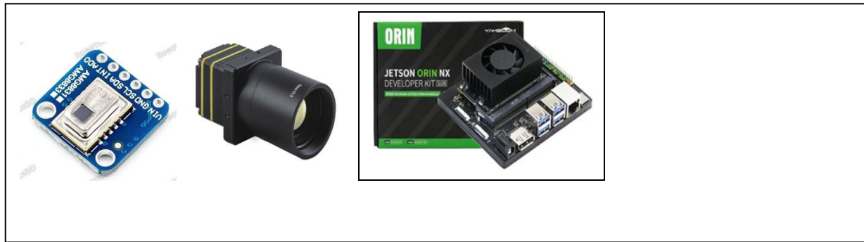
Fig. 2.7.6 Camera, Thermal Imaging sensor, and Jetson Orin NX 16GB (Ground Station)
