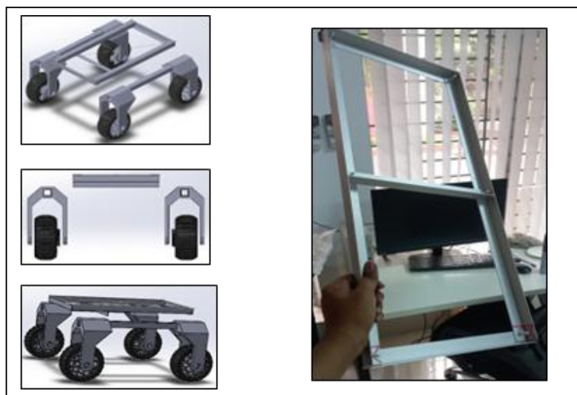
Fig. 3. CAD images of the rover chassis, manufactured chassis skeleton.
