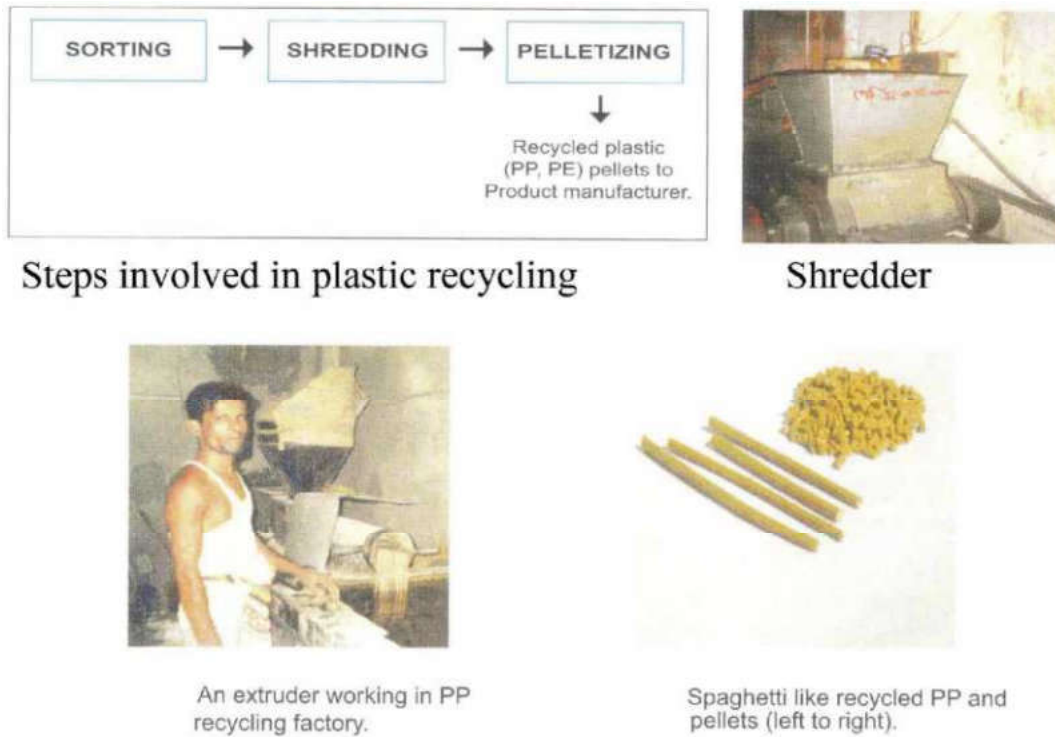
Fig. 13: Steps involved in waste plastic recycling (Islam- 2005)
