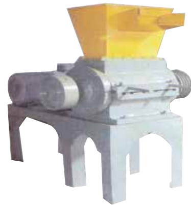
Plastic Crusher Mafia Engineering Works
