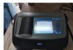
Fig. 28 spectrophotometer (Color, TSS, TDS)
