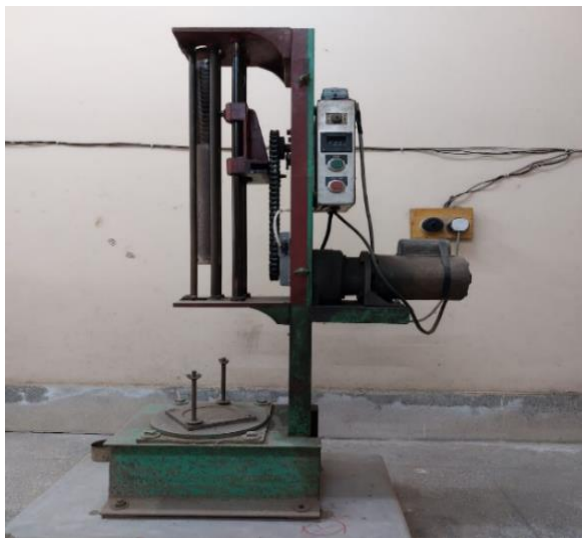
Fig. 2. Automatic soil compaction machine.
