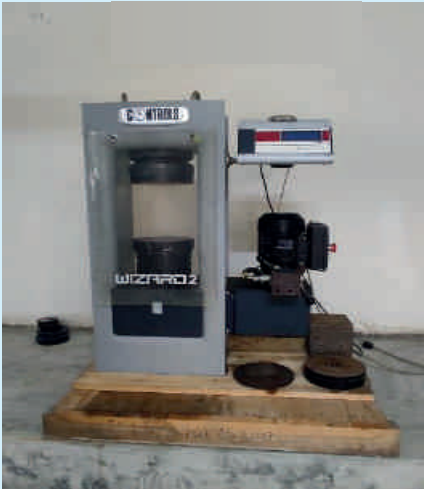
Concrete Crushing Machine
