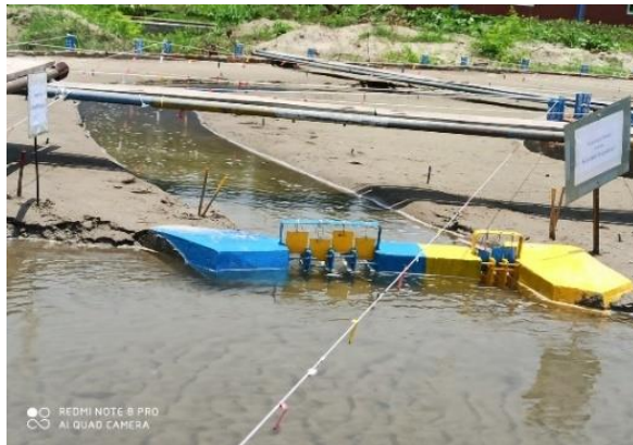
Fig. 18. Dry bed condition at and around the existing and proposed regulators in the model (T6).
