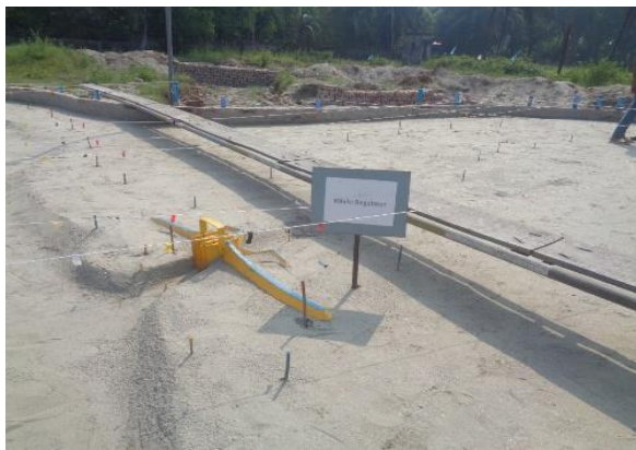
Fig. 4. Installment of Khulshi regulator in the model.
