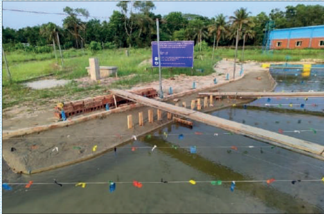
Figure: A view of the of the intake structure as reproduced in the model and flow condition at and around the proposed intake structure for bank full discharge in test T2 condition.
