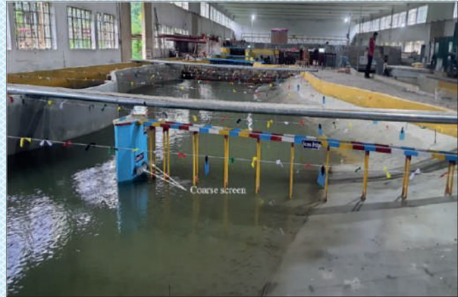
Figure: A view of the of the intake structure as reproduced in the model and flow condition at and around the proposed intake structure for bank full discharge in test T2 condition.
