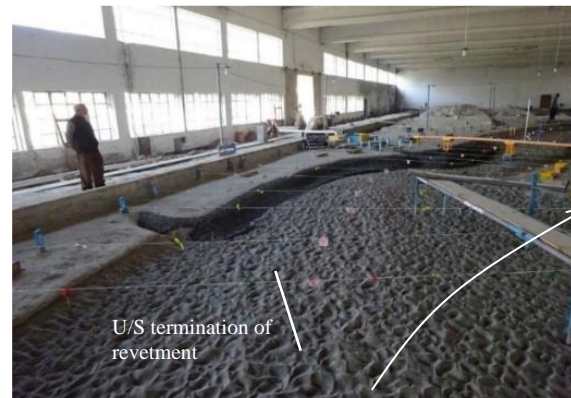
Fig. 2. U/S termination of revetment prevents the embayment due to river bank erosion (T5).
