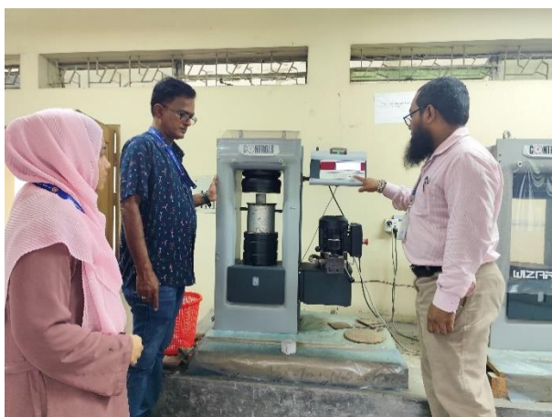
Concrete crushing machine (Controls, Italy) (left) and Core cutter machine (Hilti, Switzerland) (right) used for cutting concrete block and extract core.
