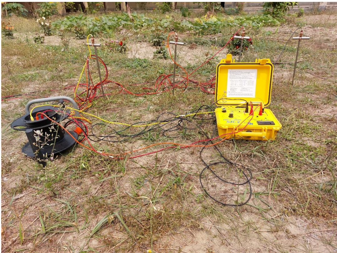
Soil resistivity meter used for sub soil investigation and ground water detection
