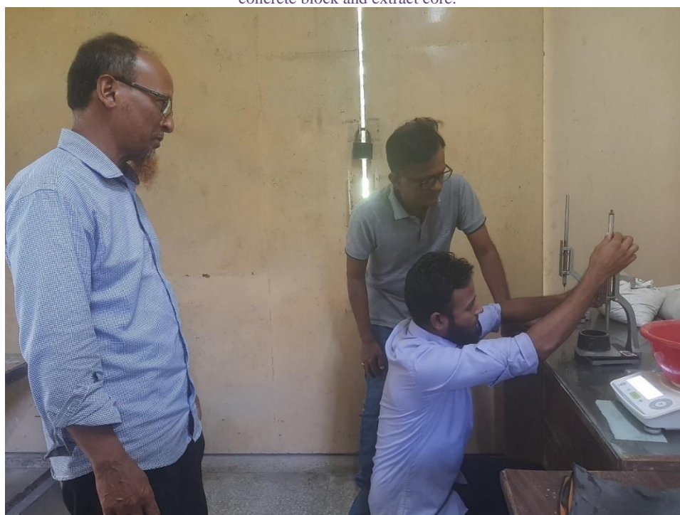
Technicians conducting consistency test of Cement
