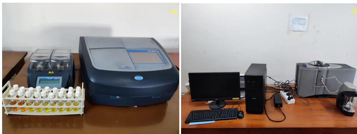
Equipment for Chemical Laboratory: (a) HACH DR 6000 Spectrophotometer & HRCH DRB 200 (b) Particle Size Analyzer (Malvern Panalytical, UK)
