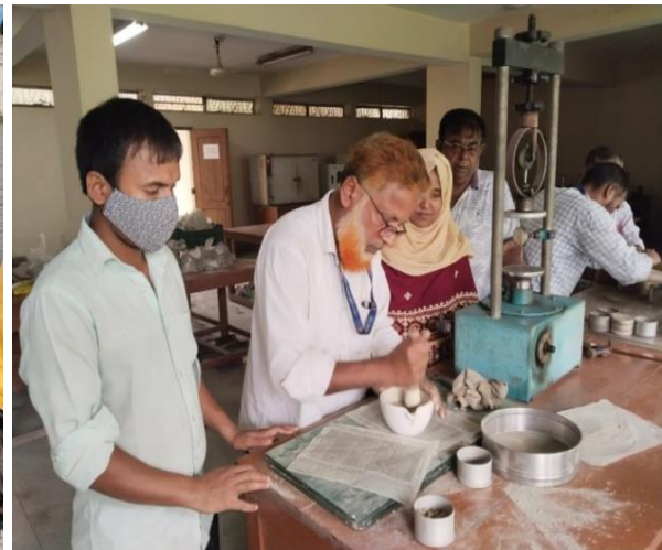
Sample collection by RRI Personnel from Palongkhali and Balukhali Khal at Ukhia & Teknaf, Cox's Bazar under Cox's Bazar O & M Division, BWDB, Cox's Bazar (left), sample preparation at RRI laboratory for Field Density and Particle Size Analysis Test (right)
