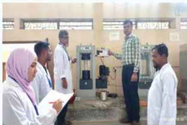
Photo: Supervision and guiding the technicians by the officer during the Compressive Strength test (left) and Cement test (right) at the Material Testing and Quality Control laboratory
