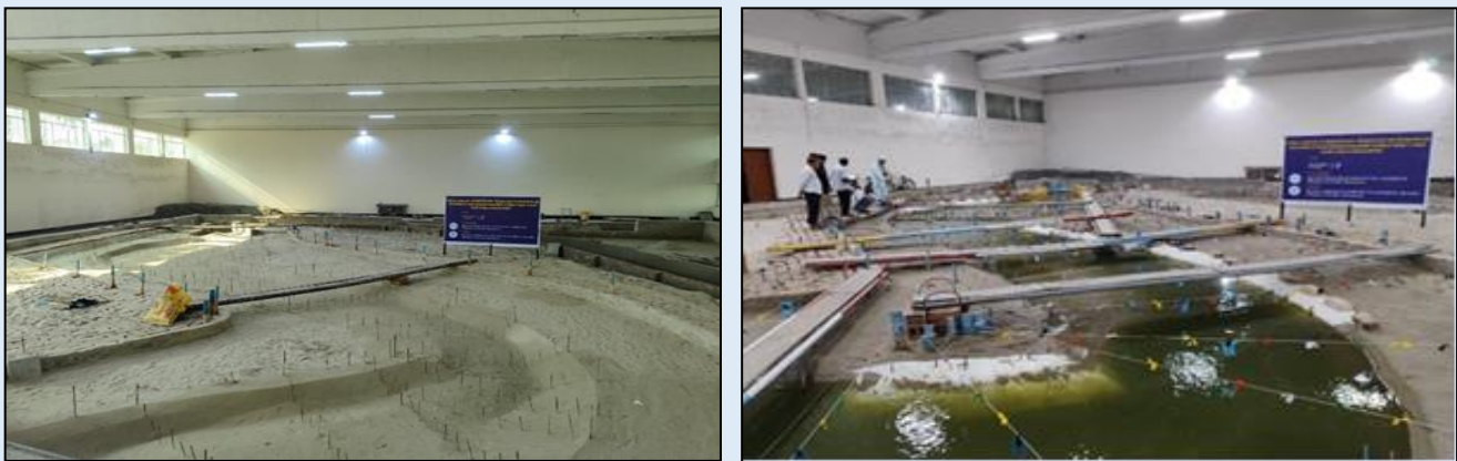
Figure: Left picture represents the model bed (before run) and right picture represents the model during running condition for the physical model in connection with Restoration and Development of Water Resources Management System of Polder 31
