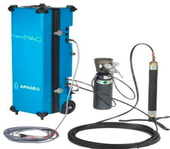
Recently procured equipment (supported by IDCB Project, Phase-II) for Soil Testing Laboratory: Menard Pressure Meter with GeoBox (Apageo, France) (left) and Hydraulic Rotary Drilling Rig (Massenza, Italy) (Right)
