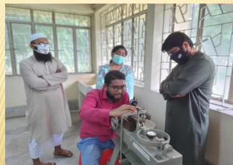
Figure-7: Running Direct Shear Test in the Laboratory
