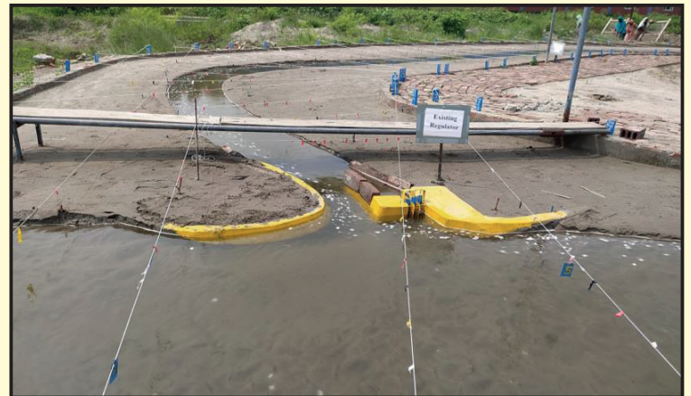
Figure (b) Flow condition at and around the regulators in test T7 for design discharge
