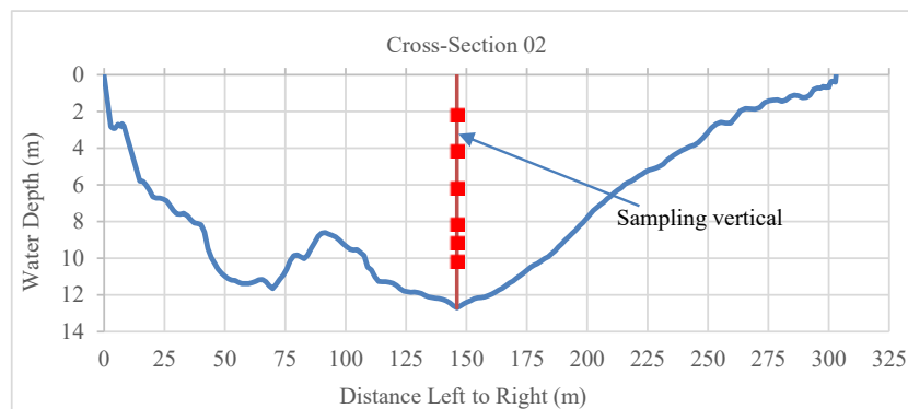
Fig. 4. Cross sectional profile (section-2)
