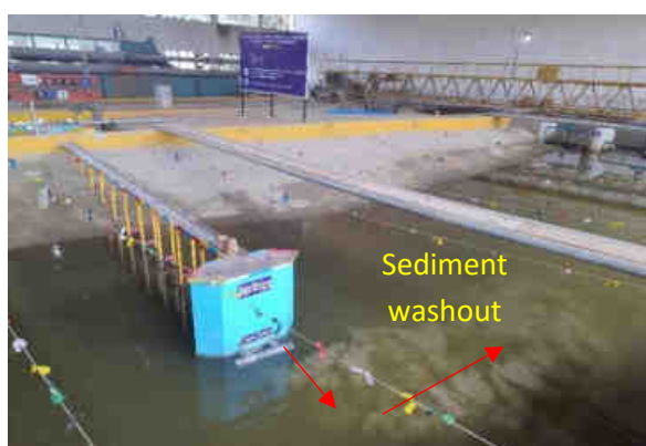
Fig. 11. Sediment washout from the distribution chamber and conveyance pipe
