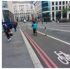
FIGURE D.2 Bollards to prevent NMT space encroachment. (London) *
