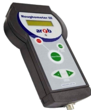
Fig-2.1: Roughometer-III (ARRB)
