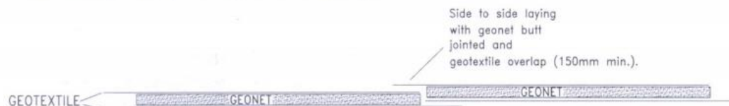
Geocomposite jointing and overlap
