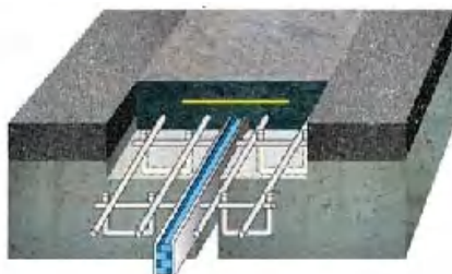
Figure 4-6 Asphaltic plug joint (left) and its surface damage (right)
