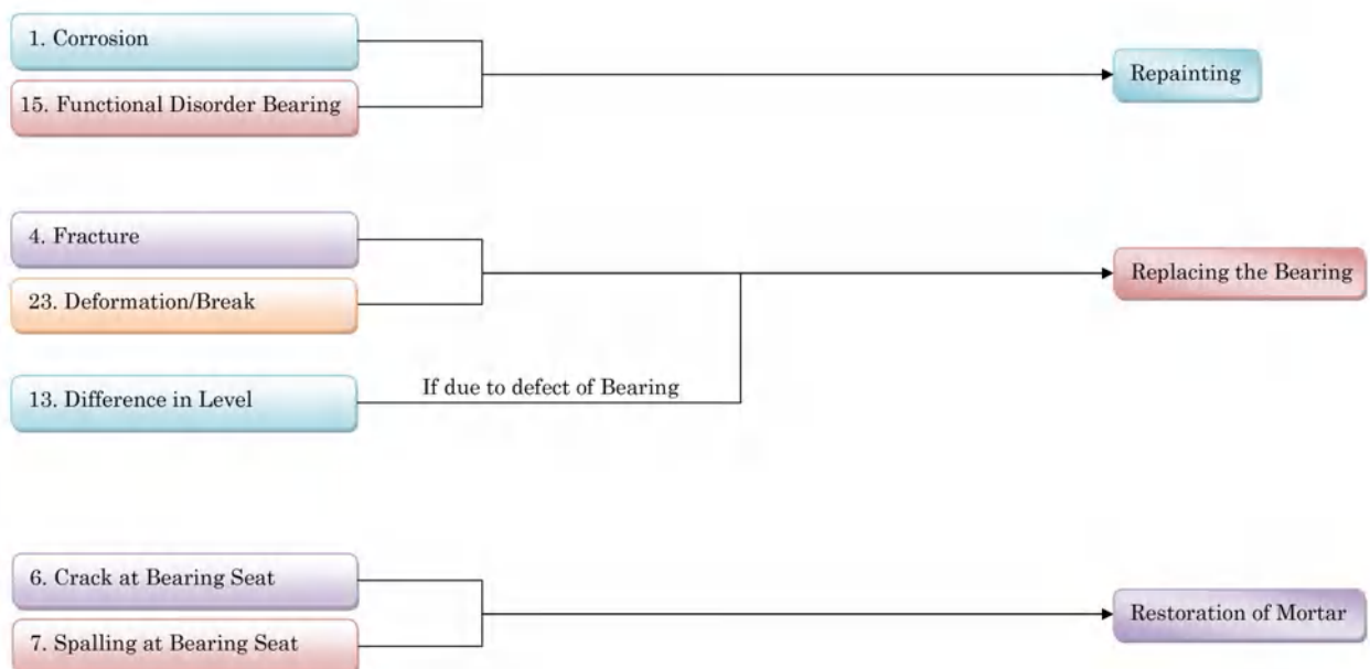
Figure 4-11 Selection Flow of Repair method of Bearing
