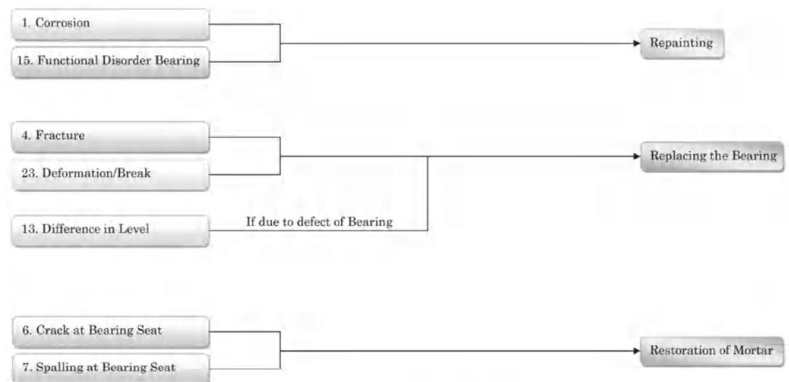
Figure 4-11 Selection Flow of Repair method of Bearing
