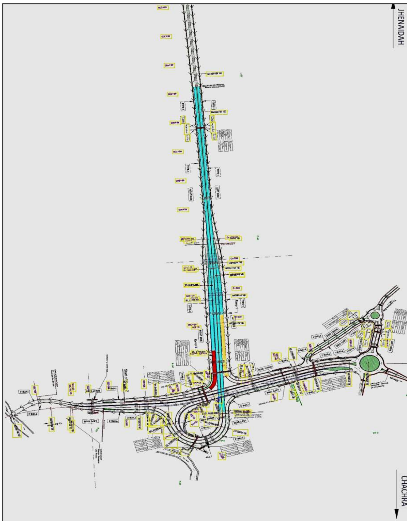
Figure 3-3: Drainage system of the proposed project area
