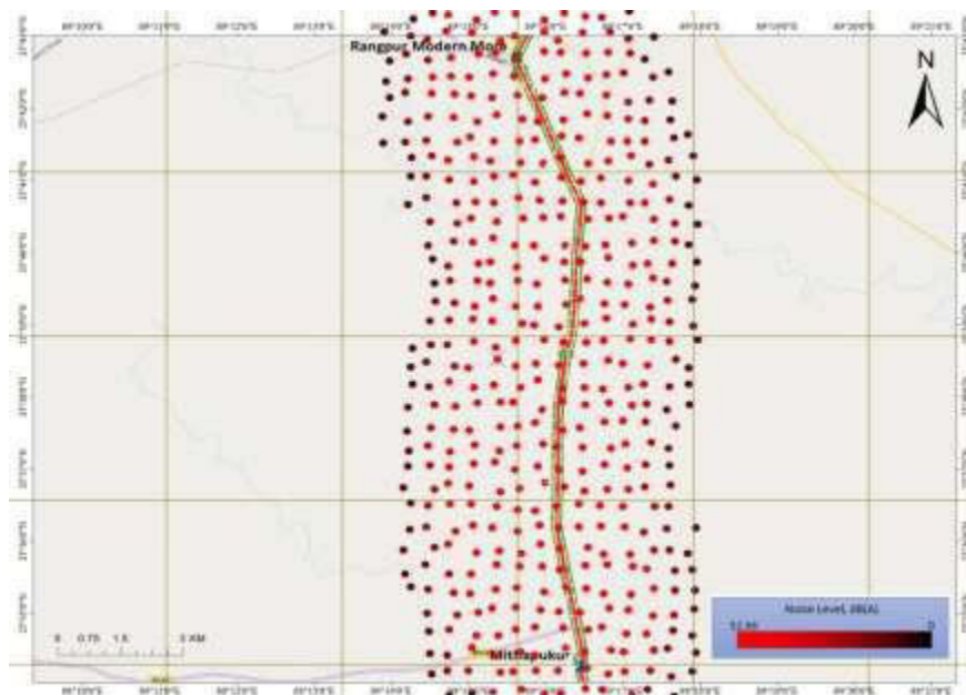
Figure G-10(b): Spatial noise intensity map of the N5-51, between Mithapukur-Rangpur Modern More, Pairabond (Box 1)
