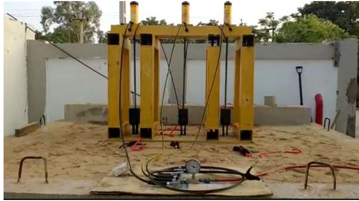
Fig 4.9-1 Typical Panel Connection Testing Setup
