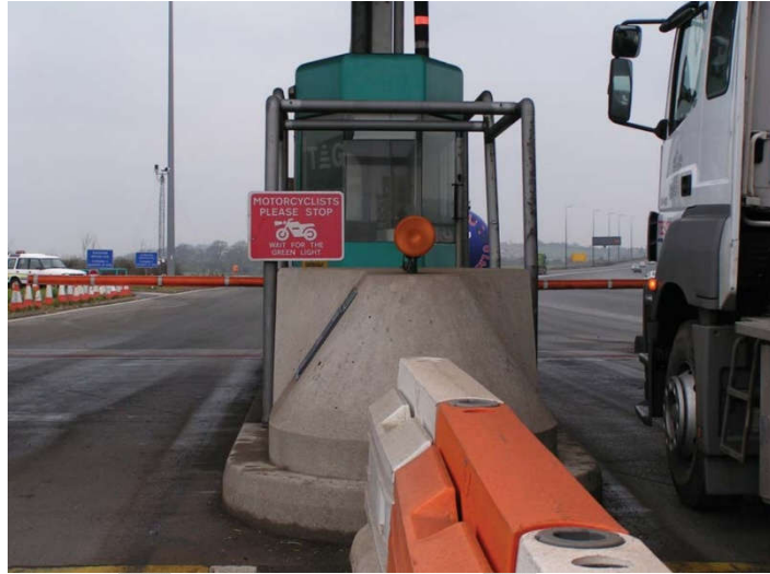
Figure 7.37-4: Use of traffic signal in front of toll booth.
