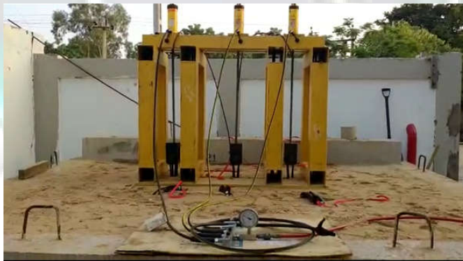
Fig 15-1: Typical Panel Connection Testing Setup
