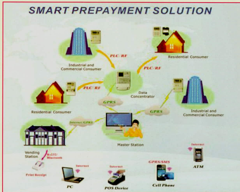
Figures: How smart pre-payment meter works
