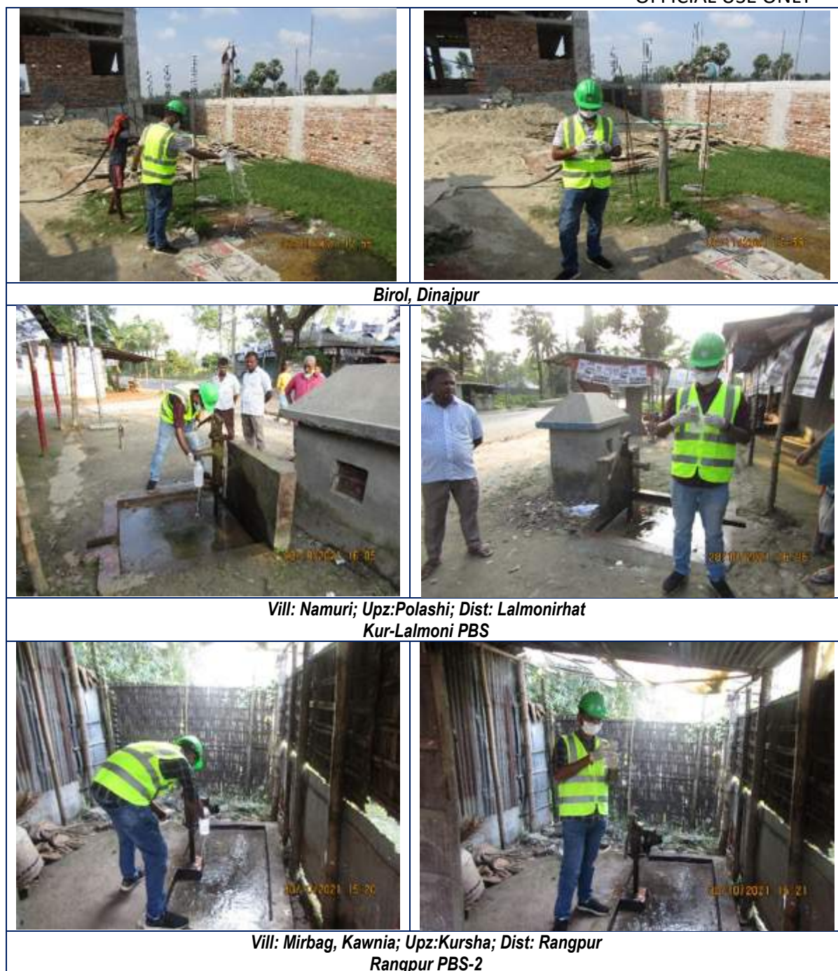
Figure IV.46: Sampling of Groundwater in the Project Area
