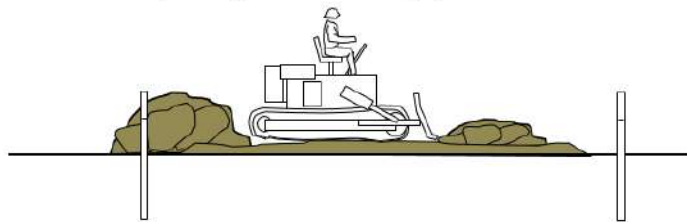
② Grading with dozer blade roughly
