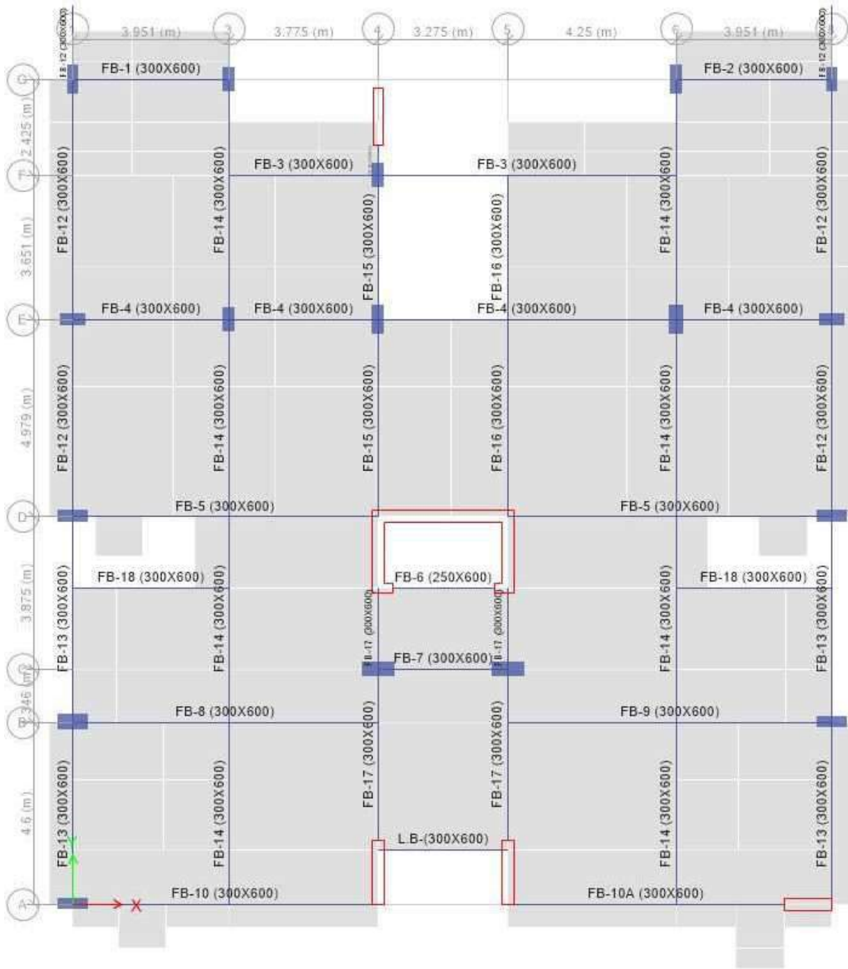
Figure A-7: Third & fourth Beam/Slab Layout
