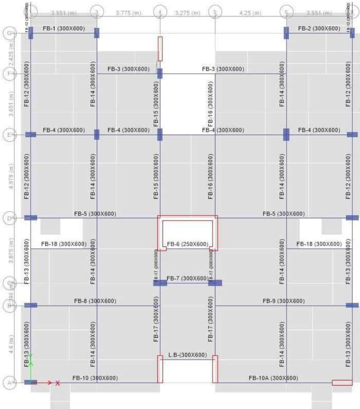
Figure A-9: Seventh Beam/Slab Layout
