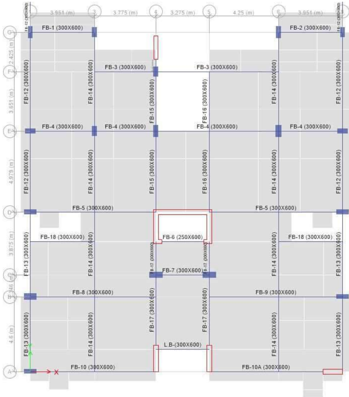
Figure A-6: Second Floor Beam/Slab Layout
