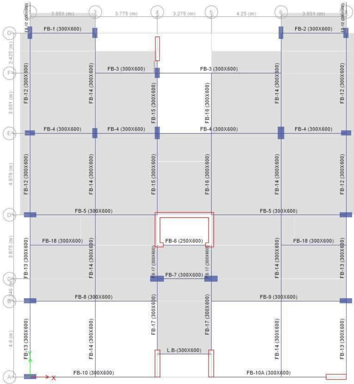
Figure C-30: Roof Floor Beam Layout
