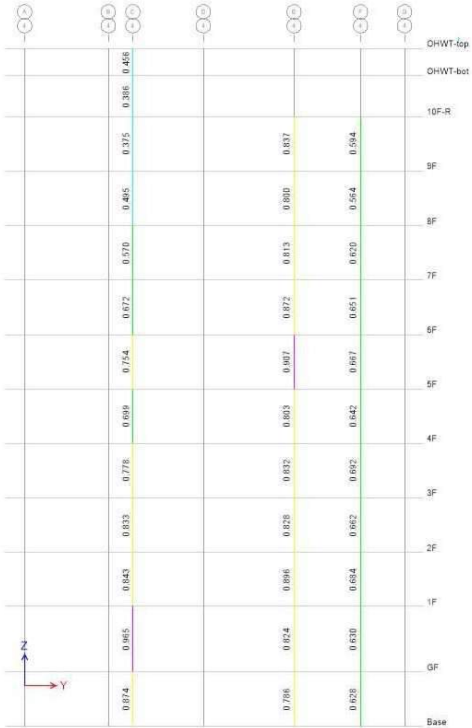
Figure C-5: Condition of Column in Grid 4
