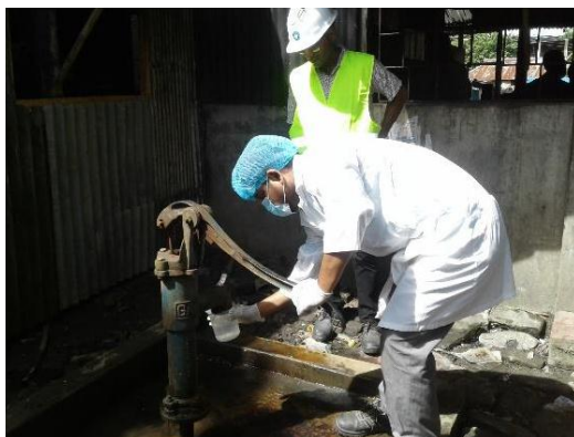
Ground Water Collection at Quasba Railway Station Tub-well Water
