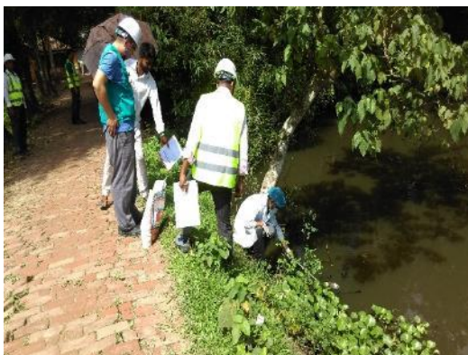
Surface Water Collection at Gonjajoori River (Down-Stream) Water
