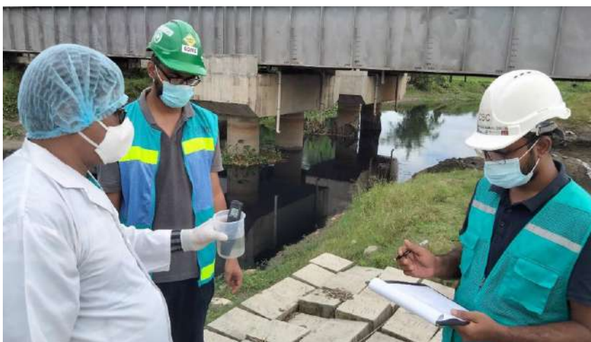
Plate 3. Surface water sample taken from Gunaiajuri station being tested for pH and TDS. Picture taken on 17 October 2021.
