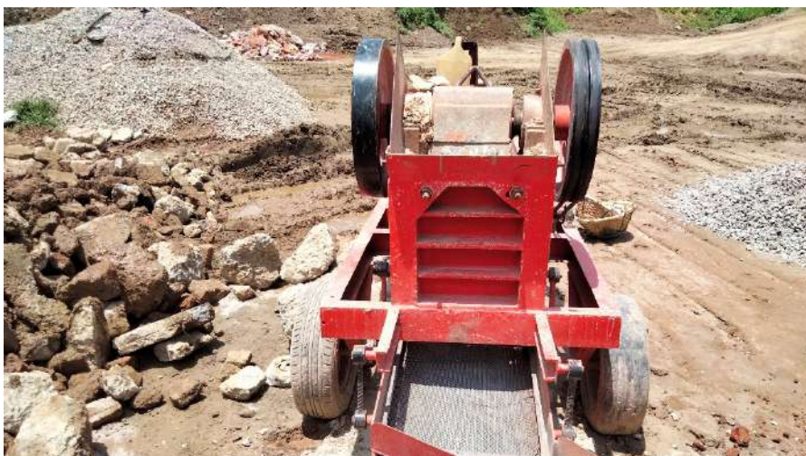
Plate 11. Photograph of a small rock crusher reducing broken concrete and other solid waste into smaller and uniform sized materials for use as concrete aggregates . Picture taken on 29 June 2022.
