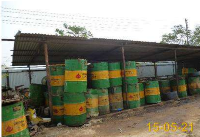
Plate 16: Used Oil drums kept under roof shed and over impermeable liner to prevent seepage to sub surface water
