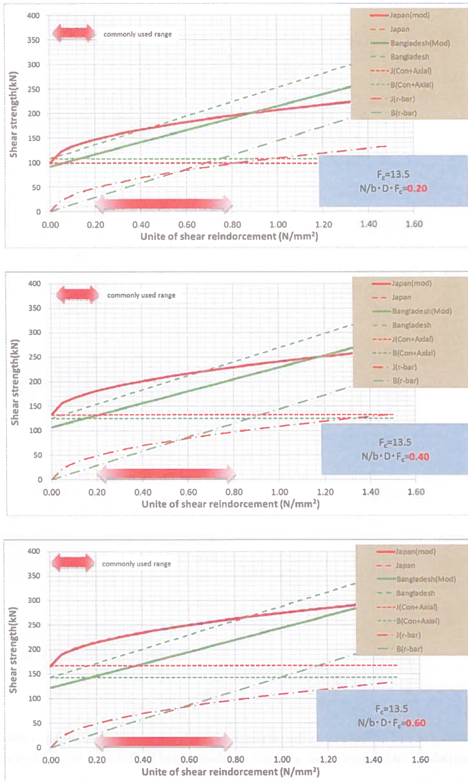
Figure S 4.6 Influence of difference in the unit of shear reinforcement on shear strength evaluation between Bangladesh and Japan (Axial force ratio is different for each graph)
