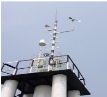
Charipara Auto Tide Gauge & Weather Station
