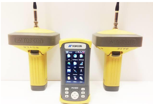
RTK Base with Topcon GPS
