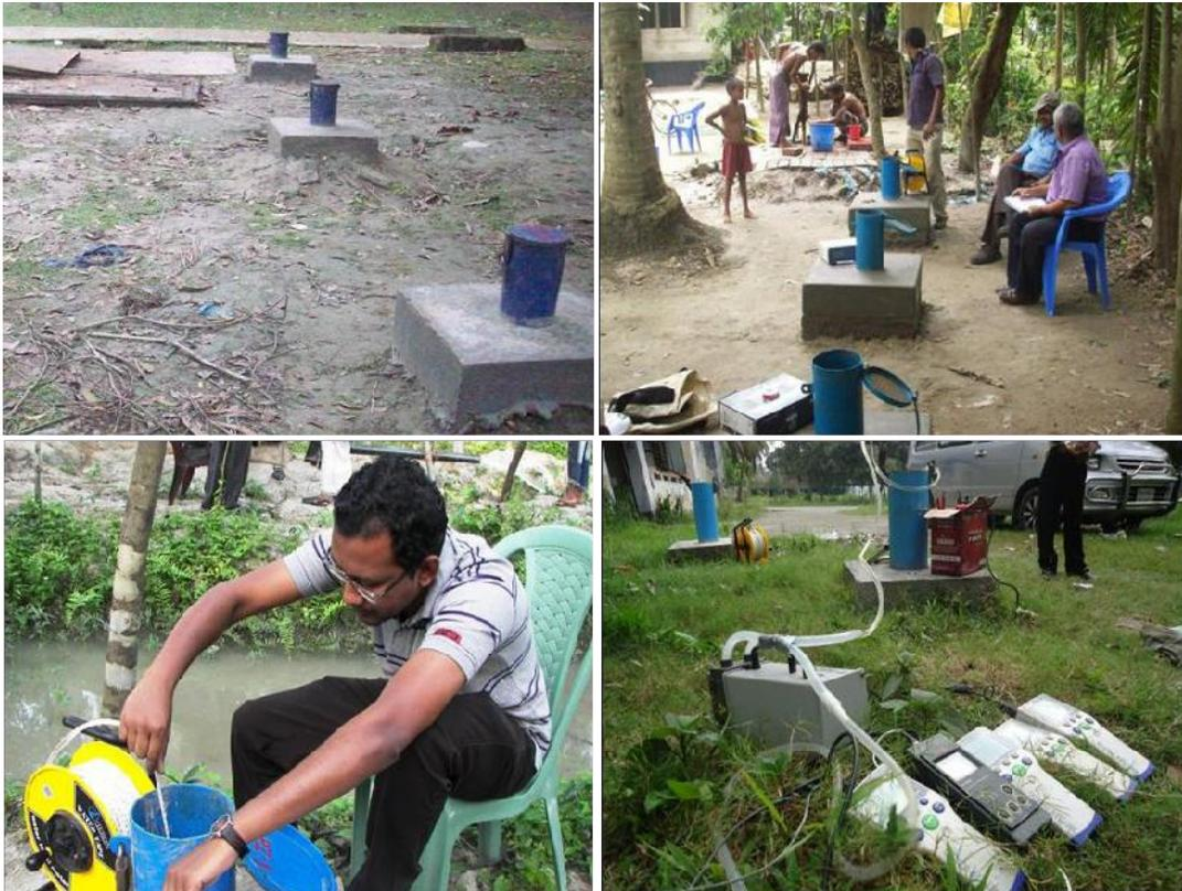
**Figure 6.8: Measurement of groundwater table and physico-chemical parameters in the field**
