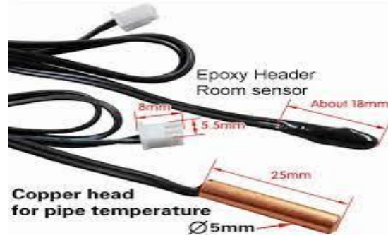
Air conditioning temperature sensor
