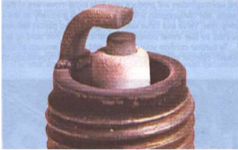
Spark plug conditions: A brown, tan or grey firing end is indicative of correct engine running conditions and the selection of the appropriate heat rating plug
