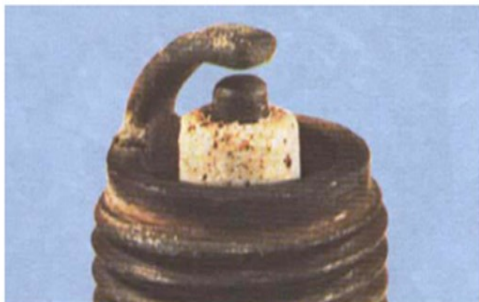
A blistered white insulator or melted electrode indicates over advanced ignition timing or a malfunctioning cooling system. If correction does not prove effective, try a colder grade plug
