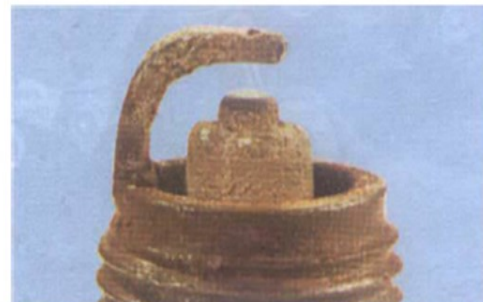
A worn spark plug not only wastes fuel but also overloads the whole ignition system because the increased gap requires higher voltage to initiate the spark. This condition can also affect air pollution.
