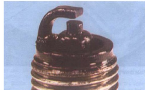
Wet, oily carbon deposits form an electrical leakage path along the insulator nose, resulting in a misfire. The cause may be a badly worn engine or a malfunctioning ignition system
