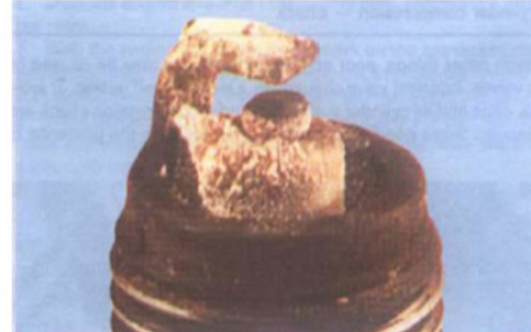
White deposits have accumulated from excessive amounts of oil in the combustion chamber or through the use of low quality oil. Remove deposits or a hot spot may form
