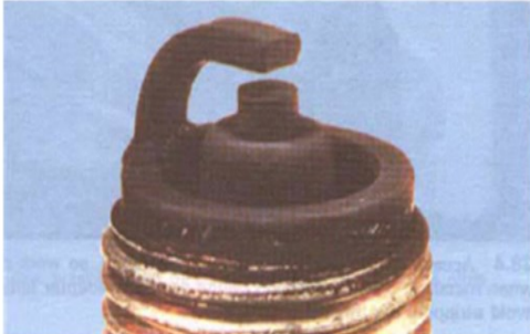
Black sooty deposits indicate an over-rich fuel/air mixture, or a malfunctioning ignition system. If no improvement is obtained, try one grade hotter plug
