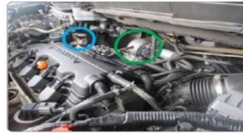
Vaporizer and LPG Solenoid, installed on a Honda CRV. Vaporizer on green, solenoid in light blue.
