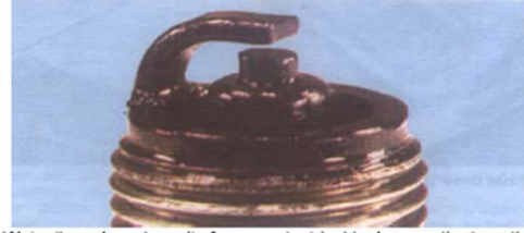
Wet, oily carbon deposits form an electrical leakage path along the insulator nose, resulting in a misfire. The cause may be a badly worn engine or a malfunctioning ignition system
