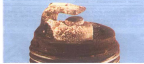
White deposits have accumulated from excessive amounts of oil in the combustion chamber or through the use of low quality oil. Remove deposits or a hot spot may form
