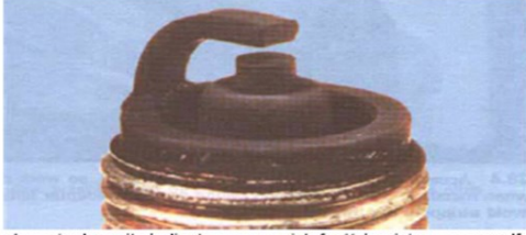
Black sooty deposits indicate an over-rich fuel/air mixture, or a malfunctioning ignition system. If no improvement is obtained, try one grade hotter plug
