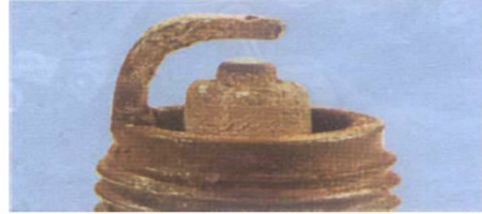
A worn spark plug not only wastes fuel but also overloads the whole ignition system because the increased gap requires higher voltage to initiate the spark. This condition can also affect air pollution.
