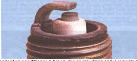
Spark plug conditions: A brown, tan or grey firing end is indicative of correct engine running conditions and the selection of the appropriate heat rating plug
