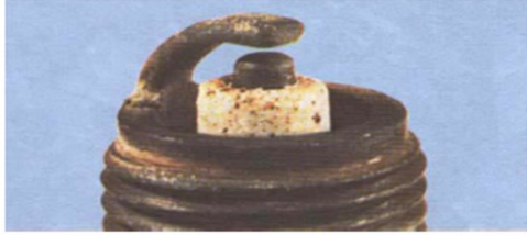
A blistered white insulator or melted electrode indicates over advanced ignition timing or a malfunctioning cooling system. If correction does not prove effective, try a colder grade plug
