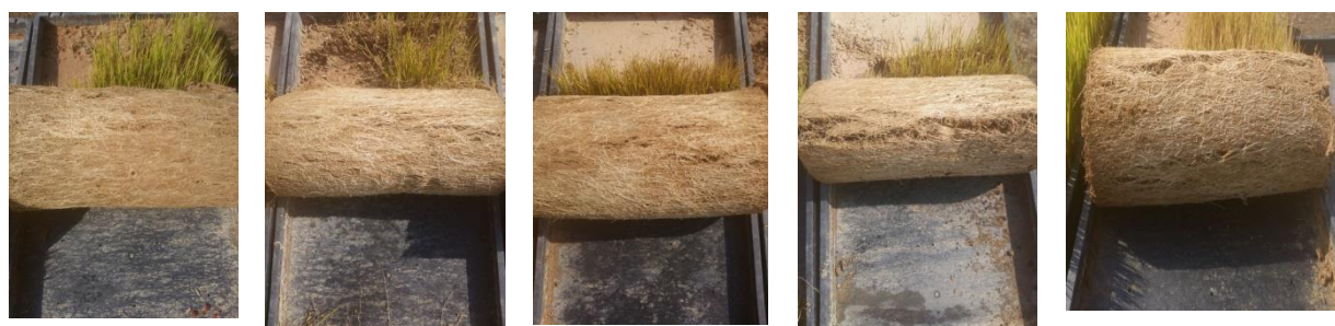
1: 100% soil (zero tea wastage) 2: 95% soil (5% tea wastage) 3: 90% soil (10% tea wastage) 4: 85% soil (15% tea wastage) 5: 80% soil (20% tea wastage)
