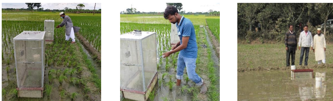
Fig. 26. CH 4 , N 2 O and CO 2 collection from rice fields
