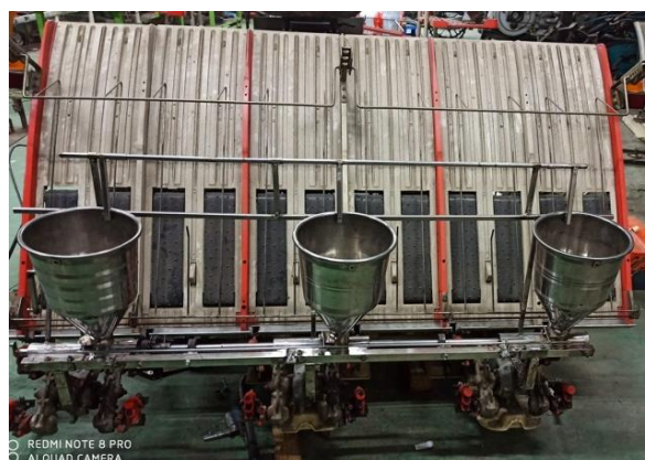
Fig. 28. Rice transplanter cum fertilizer applicator (Riding type)
