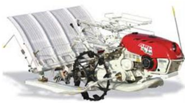
Fig. 1. Walking type rice transplanter (South Korea and ARP-4UM)
