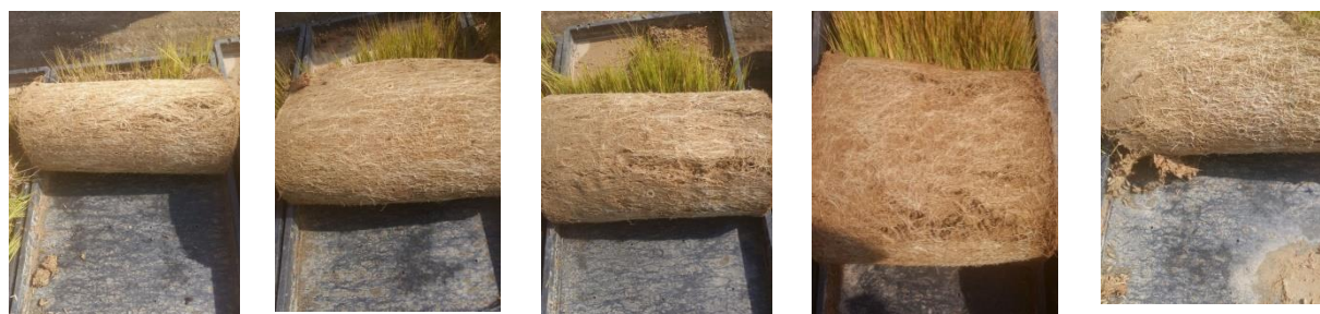
1: 100% soil (zero rice husk) 2: 95% soil (5% rice husk) 3: 90% soil (10% rice husk) 4: 85% soil (15% rice husk) 5: 80% soil (20% rice husk)
