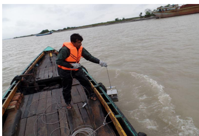
Sampling of RBM_03 and Ben_03 using Eckman Dredger at Shalobunia dated 25/07/2015 at 10:15 AM
