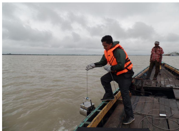
Sampling of RBM_01 and Ben_01 using Eckman Dredger near the Power Plant site dated 25/07/2015 at 12:40 PM
