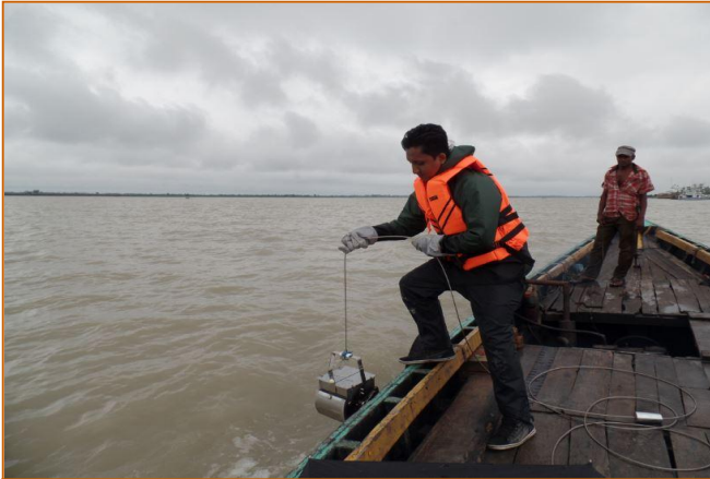
Sampling of RBM_01 and Ben_01 using Eckman Dredger near the Power Plant site dated 25/07/2015 at 12:40 PM
