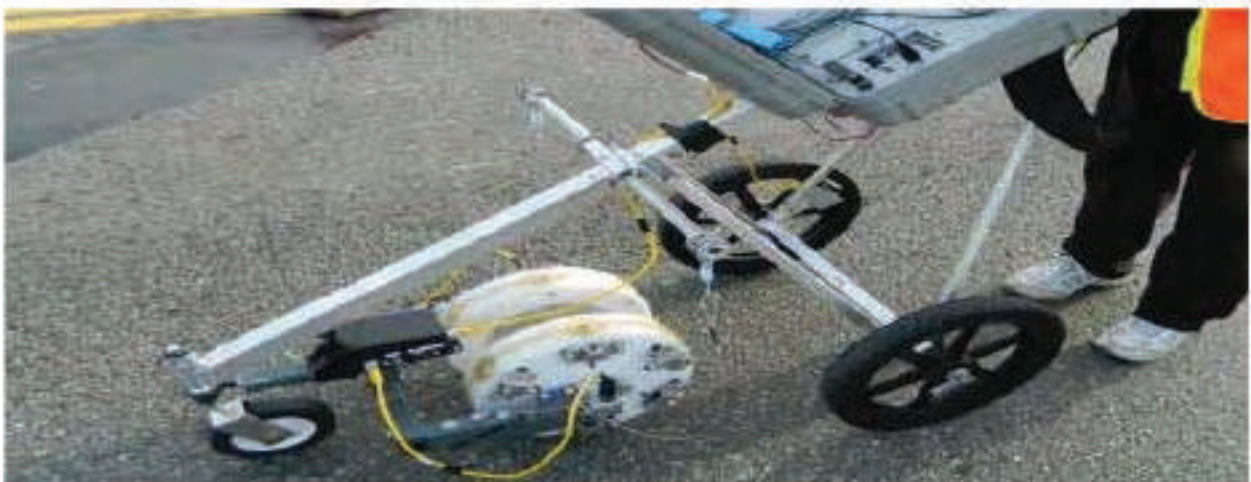
Figure 6.19: Impact Echo Testing
