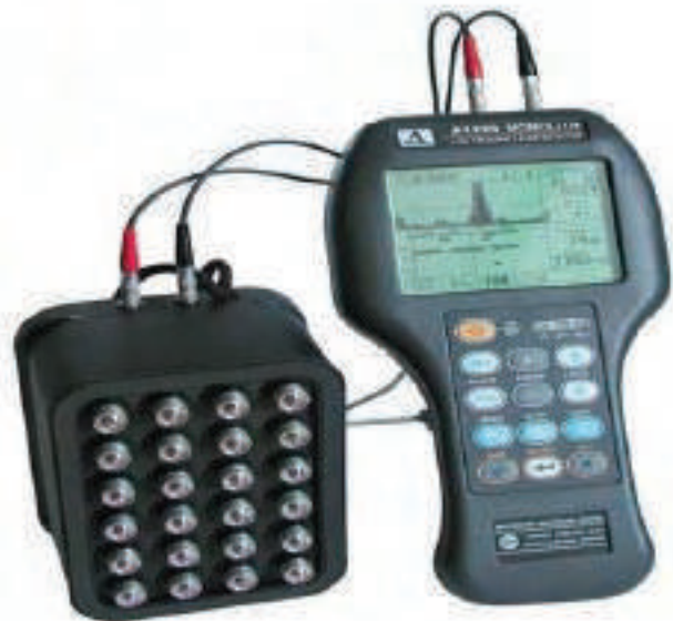
Figure 6.21: Ultrasonic Echo Control Unit and Sensor Array
