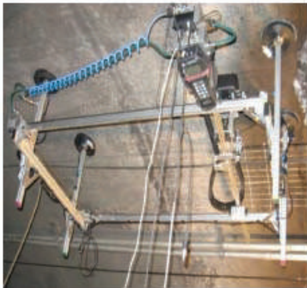
Figure 6.20: Ultrasonic Echo Control Unit Mounted on Automated Scanning Device
