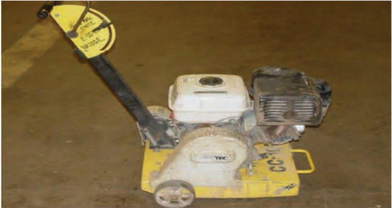
Figure 7.2: Crack Router for Preparing Horizontal Cracks
