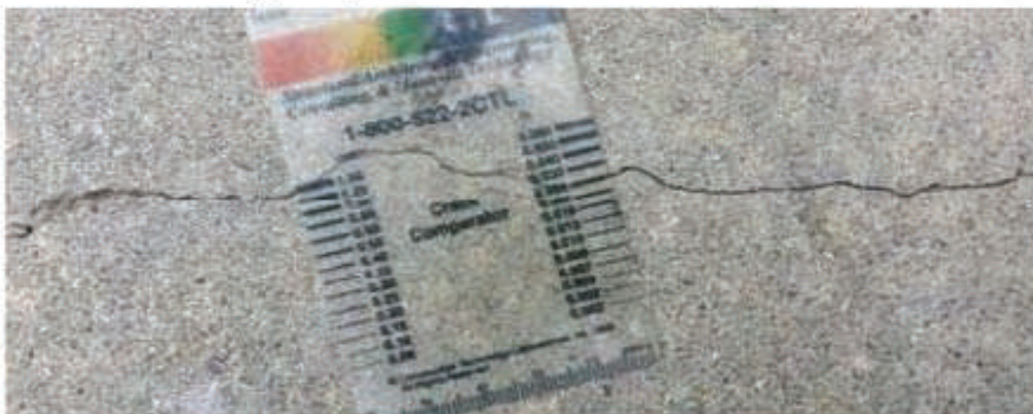
6.11: Crack Comparator for Determining Crack Width
