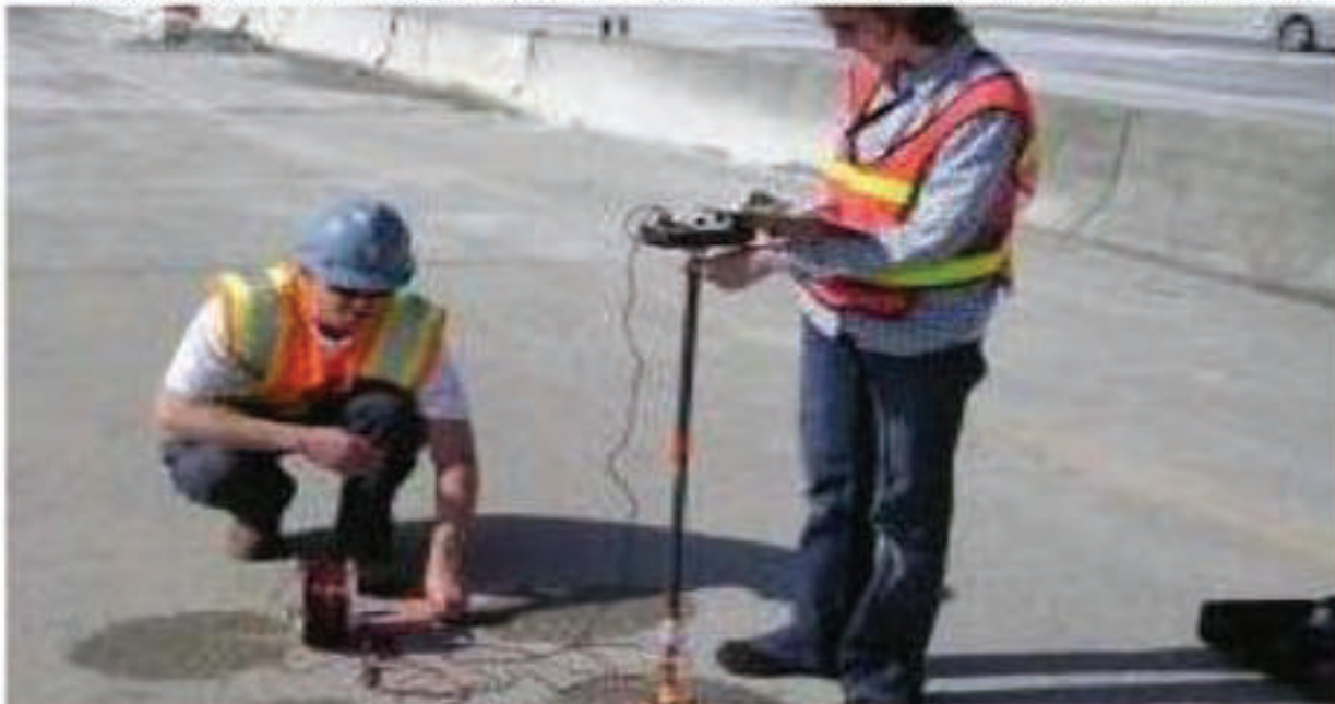
Figure 6.14: Example of Half-Cell Potential Test
