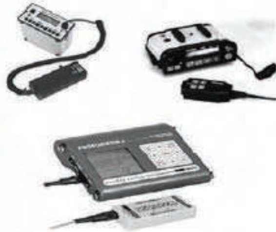
Figure 6.16: Examples of Pachometer Equipment
