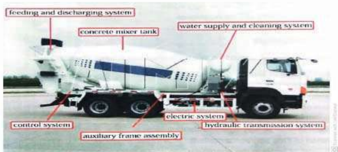
Concrete mixture truck
