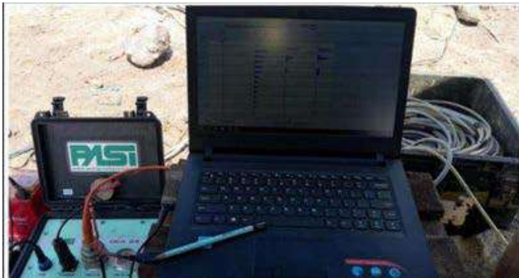
Figure 8-1: Downhole Seismic Test data logger
