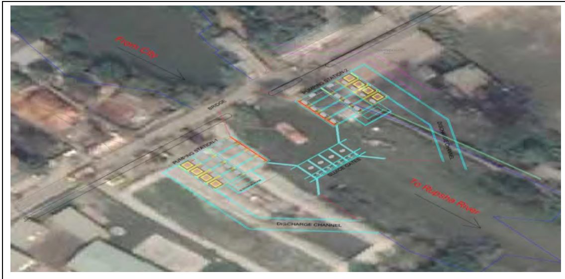
Figure 3.35 Labonchara Gate and Pumping Station Layout Options
