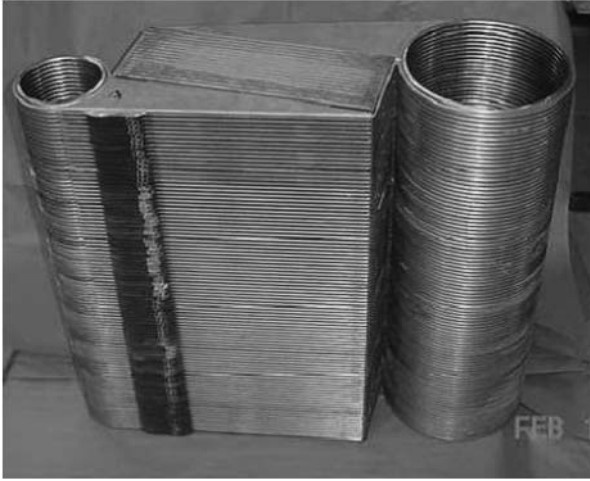
Figure 11-5. Courtesy of Ingersoll-Rand Energy Systems. The recuperator is integral with the combustor (not shown) thereby eliminating transition parts. The combustor fits into the large circular chamber on the right side of the photograph and is mounted directly above the compressor-turbine components.
