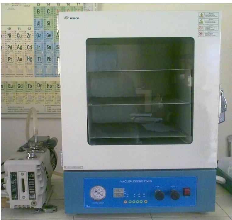
Used for the drying of samples in vacuum condition.
